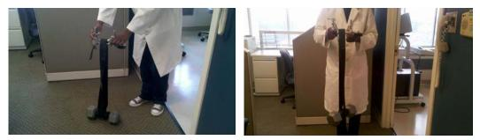
Average the three calibration trials. The dynamometer should be accurate within  $\pm 2$  kgs for the average of the three calibration trials. If the result is outside the  $\pm 2$  kg range after following the Troubleshooting tips below, you must send the dynamometer to the manufacturer for repair and recalibration. **DO NOT attempt to recalibrate the dynamometer yourself.** Calibration problems can be caused by dropping the dynamometer or by leaks in the hydraulic system.
