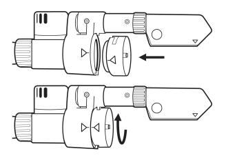
Insert the barriette<sup>™</sup> in the one-way valve (aligning the arrows) as shown below. Check that it sits tight.
