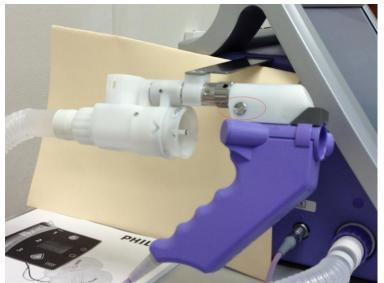
The picture below shows the purple hand sensor after you have removed the white motor block
