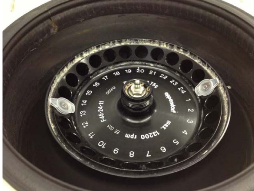
Figure 89: Example of centrifuge tube counterbalancing placement
