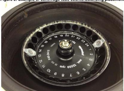
Figure 9: Example of centrifuge tube counterbalancing placement
