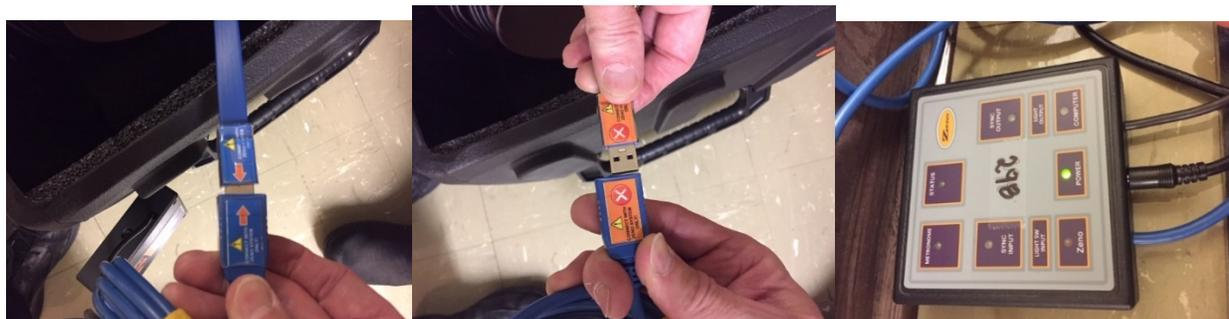
When connected successfully, only the green light above the "Power" button will be on.
